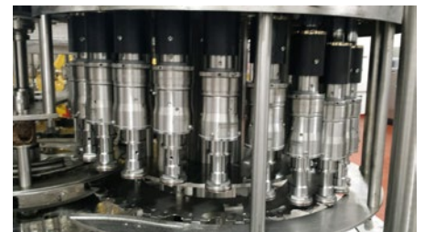
Zalkin Conversion from Gripper Chuck to one piece chuck for Gatorade
