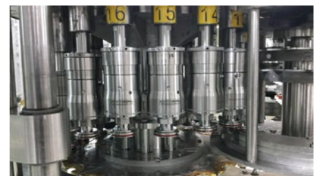
Capper Clutch & Chuck on Krones 24 Head Capper
